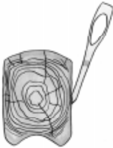
1900 Model (Most Common) Double-sided Sharpening for all types of hewing of timber and corner chopping "Chopping Broad Axe"
